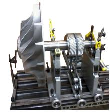
■HOFMANN BALANCE MACHINE. Rely on our balancing experts for accuracy in analyzing your equipment problems using this balancer. We can balance to any certification: API, ISO G2.5, SAF/ARP, etc.
